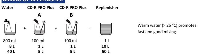
Mixing time: approx. 1 minute, after every addition of Part A and B, as well as for ready prepared replenisher. Only as much replenisher should be prepared, as will be used up within 1-2 weeks. The tank must be covered and protected from access of air.
